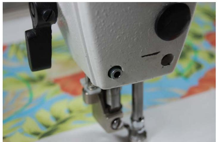
*3. Take the longer black screw that is supplied with your handles and put a small washer on it. Insert into the empty screw hole on the Voyager and get it started with the allen wrench that is supplied. Don't tighten it all the way down yet, just get it started about halfway.*
