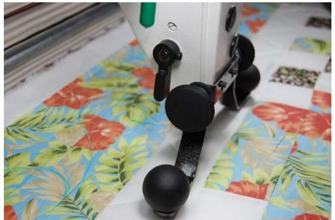
You can also mount the handles with the u-shaped bracket facing toward you. This means the handles are in front of your machine a little bit, but you will be able to move your presser foot lever forward or back, and the handles are totally clear of the pigtail thread guide.
