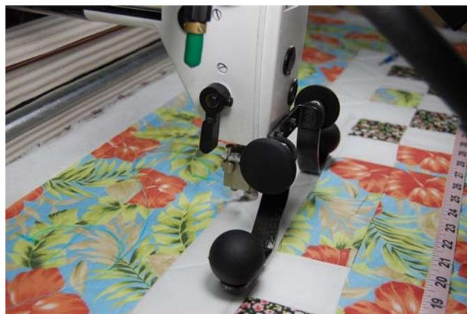
*The handles are also adjustable. They can be raised up if they are too low to your quilt or you happen to be using thicker batting or quilting on a quilt with trapunto. Simply unscrew the top, flat knobs, twist off the collar and washer, slip the handle off (leaving the rubber washer on the peg), and reattach in the lower hole on the arm. Now reattach the collar, washer, and knob in this order.*
