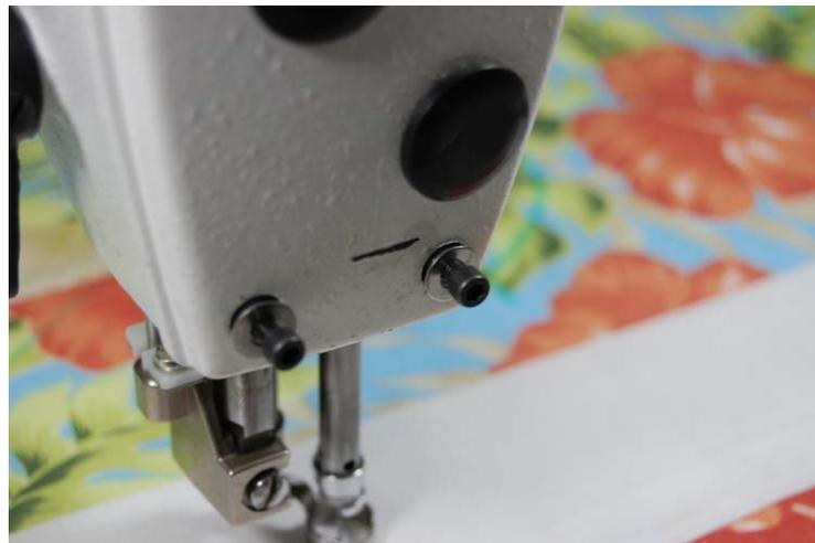
5. Slide the bracket over the screw heads, making sure the washer on the screw is behind the bracket and against the machine. Drop the handles down into the slots on the bracket and make sure they're seated down in and level...
