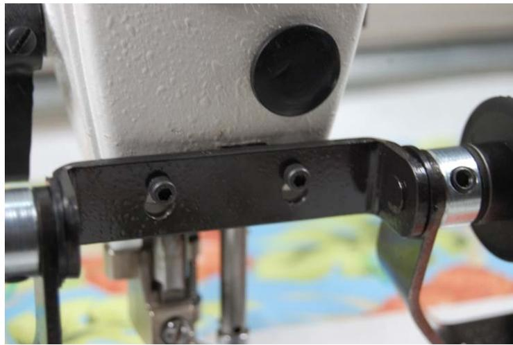
6. Now tighten down with the allen wrench a little bit at a time on each side, making sure the handles stay seated down in the teardrop-shaped holes on the bracket. (Don't tighten one side all the way down before tightening the other side... alternate back and forth so it's even.) Make sure you tighten the bracket until it is tight against the machine, but do not over tighten.
