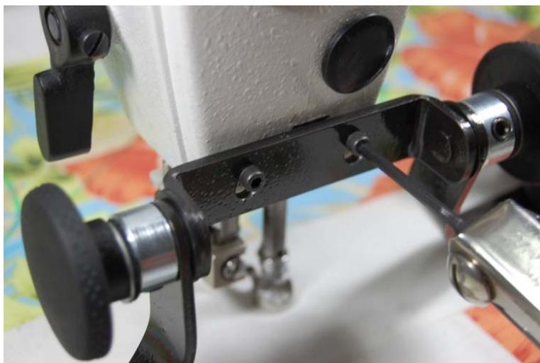
7. If you ever need to completely remove your handles, just loosen the screws with the allen wrench a little bit and slide the handles up and off... Then retighten the screws to hold your cover snug. No need to take these screws back out unless you need in the front of your machine.
