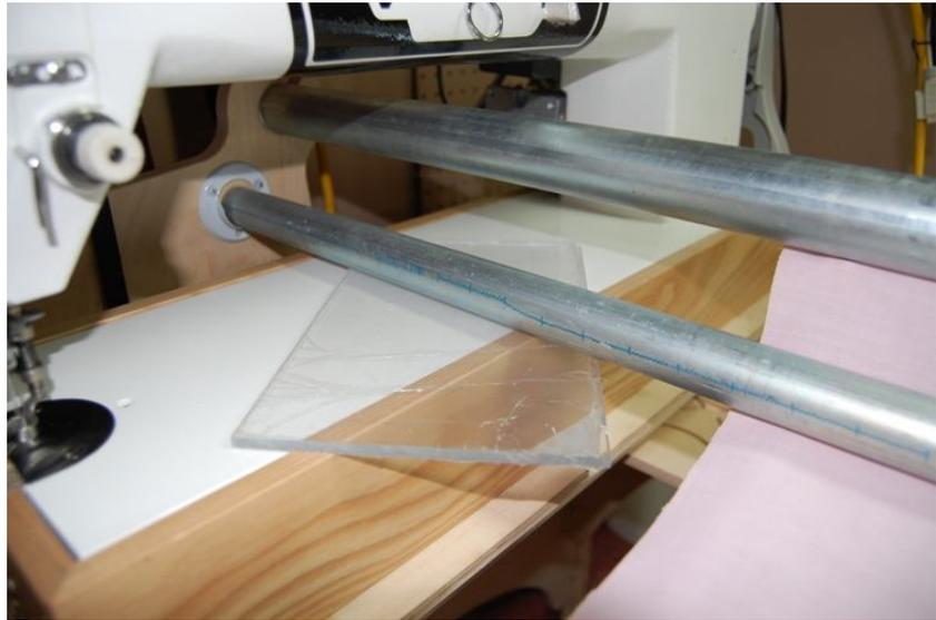
Slide the brackets on the bar and lay the bar through the machine and on top of something that is 1/2" high... (like I said, I used 2 pieces of plexi-glass on top of each other) Two 1/4-inch thick longarm templates/rulers would work....
