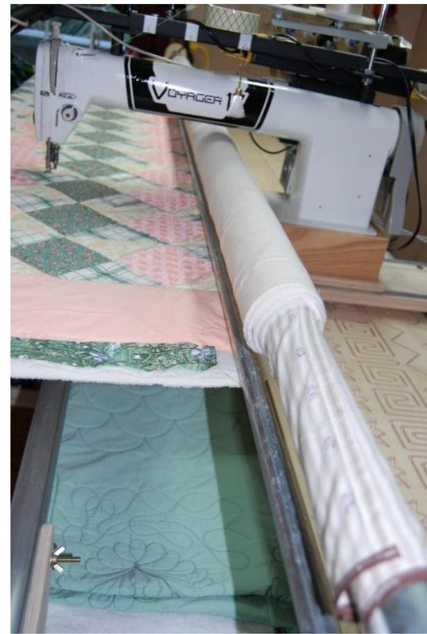
Once you have your bar back as far as you can without it hitting the cogwheel, screw that bracket down with at least 2 screws so it doesn't move... You might have to have someone lift the take-up roller out of its slot to get a screwdriver in there... Measure how far in the edge of the bracket is from the back of the arm...
